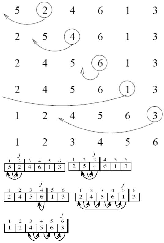
Best case: the inner loop is never executed Worst case: the inner loop is executed exactly j - 1 times for every iteration of the outer loop
