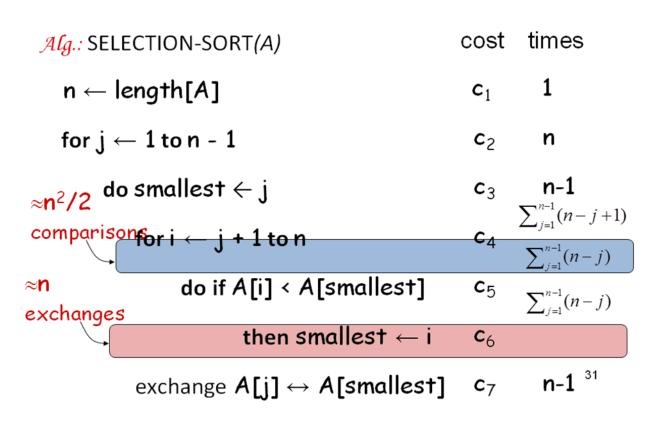
$$T(n) = c_1 + c_2 n + c_3 (n-1) + c_4 \sum_{j=1}^{n-1} (n-j+1) + c_5 \sum_{j=1}^{n-1} (n-j) + c_6 \sum_{j=2}^{n-1} (n-j) + c_7 (n-1) = \Theta(n^2)$$
